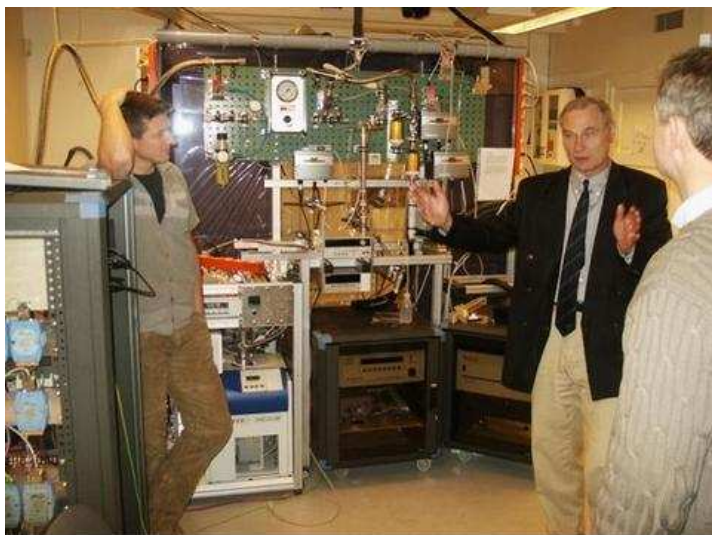
Figure 7: The Danish National Space Center SKY reaction chamber experiment. The experiment was built with the goal of pinning down the microphysics behind the cosmic ray/cloud cover link found through various empirical correlations. From left to right: Nigel Marsh, Jan Veizer, Henrik Svensmark. Behind the camera: the author.
